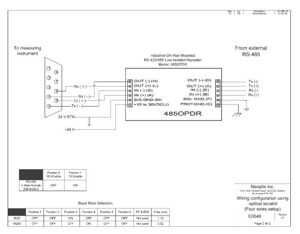
These modules are DIN rail mounted. And external DC power supply is required (+24 V on the above drawings); we recommend that you use the same power supply as for the T/Guard system (18 to 24 VDC).
