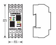
The Xpress DR model should have a serial connection as shown here (RS485, 2W and 4W). Make sure also that the little red switch RS232-RS485 is in the RS485 position.
