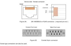
If an RJ45 or a 9-pin D-shell connector is used for a standard MODBUS device, the pinouts hereafter must be respected for every implemented circuit.
