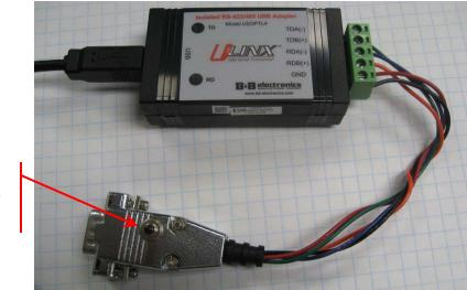
Switch (Press during power up to disable Modbus mode)
